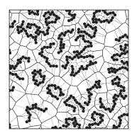
A Voronoi diagram for N=16 and  $\varphi_m=0.2$ . Filled circles represent monomers. Solid and dashed lines represent connected and disconnected edges of polyhedra, respectively.
